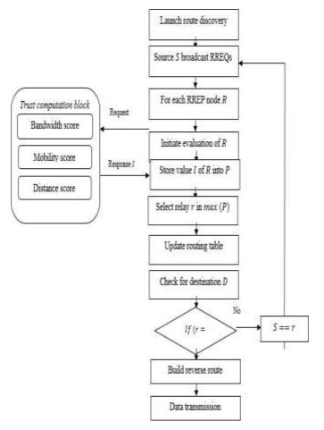
Figure 3.1 Architecture of proposed route discovery algorithm
